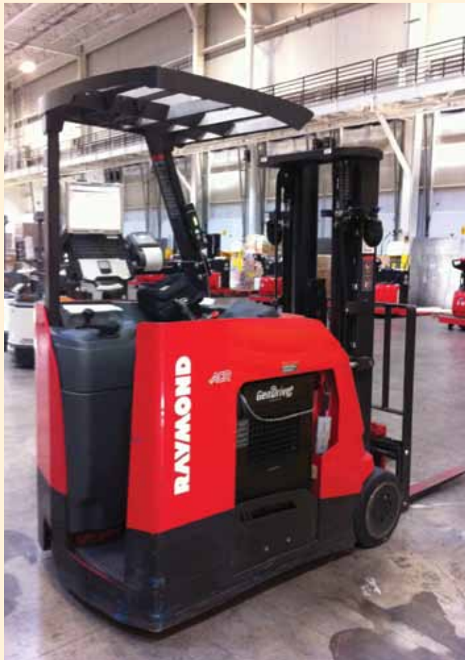
One of the fuel-cell-powered forklifts being used at the Wegmans Retail Service Center.
